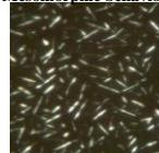
The texture of the Iso-SmA\* phase transition on cooling at about 155°C. (Planar alignment; cell thickness is 2  $\mu\text{m}$ ; width of the microphotograph is about 200  $\mu\text{m}$ ).
