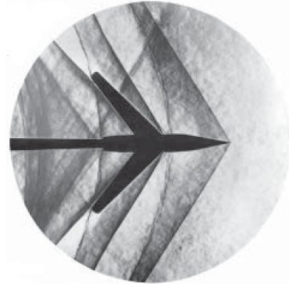
Fig.1: wave drag on the surface of the aircraft
